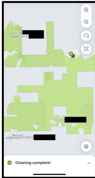
Screenshot from the iRobot Home app interface showing, among other things, the ability of iRobot devices to detect the presence of other smart devices connected to the same WIFI network (as well as their (partial) MAC addresses).
